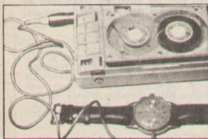
Watches have ears: the miniature mike inside leads to this coat-pocket recorder
